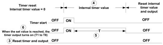
T= timer set value **OFF OFF** ON ON ON **OFF** Timer start 6 OFF **OFF** ON When the set value is reached, the timer output turns on (T1 to T8) ON OFF (3) Reset timer and output OFF
